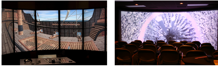
Figure 1: Tiled LCD immersive environment (left) and Continuous immersive system (right).
